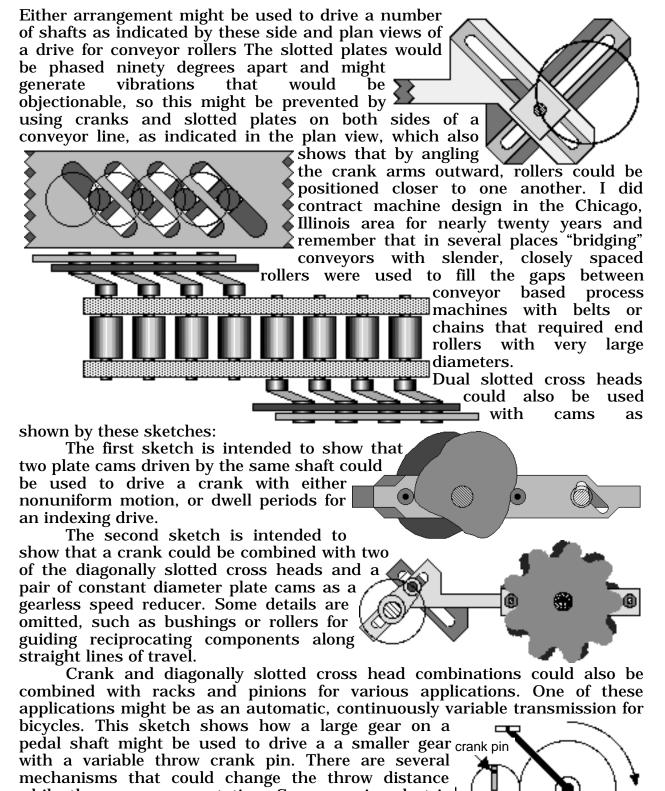
while the gears were rotating. Some require electric motors, so it might be better to use a mechanism that could be actuated manually, or perhaps in response to increased loading of the type that occurs when a bicycle starts up a hill.
