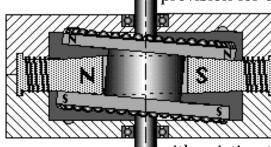
but this could be provided by using the wobble gear as a rolling switch that would sequentially connect an annular conductor embedded conductive to segments connected to two or more windings similar to the field winding shown in this sketch.
