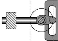
motion of a crank into sinusoidal reciprocating motion that can't be provided by using a connecting wrod to couple a crank to a reciprocating component such as a piston. They haven't been used much for <sup>©</sup> converting reciprocating motion into rotary motion, possibly because of the "dead center" problem indicated by this sketch.
