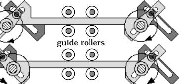
shown in some of these sketches. A useful feature of these drives is that slotted crossheads coupled with slots parallel to one another would drive cranks in the same directions, while crossheads with their slots perpendicular to one another would rotate in opposite directions. Applications that required greater degrees of precision or durability than the rubbing contacts of crank pins and slots provide might use ball bearing bushings, as indicated in the next sketch.
